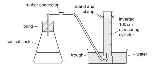
Using a measuring cylinder,  $50 \, \text{cm}^3$  of dilute acid **X** was poured into the conical flask. 0.5 g of magnesium ribbon was added to the conical flask and the bung added.
